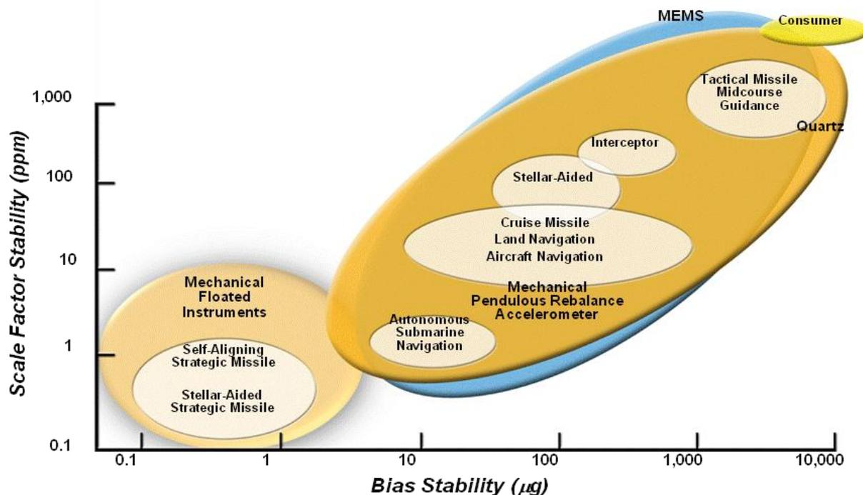
Figure 6. Current Accelerometer Technology Applications.
