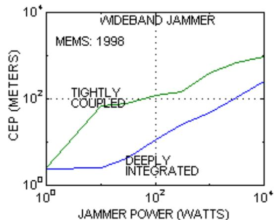
Fig. 17 CEP versus wideband jammer power.
